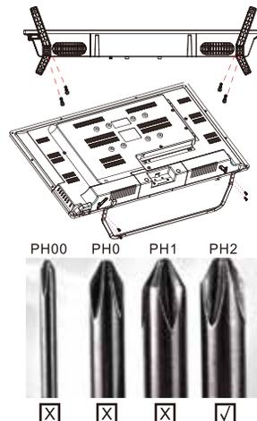
To make it more convenient for base installation and to avoid any risk of scratches and damage, we advise you using the type of PH2 screwdriver.
