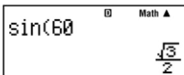
Calculator display showing  $\sin(60)$  and the result  $\frac{\sqrt{3}}{2}$ . The display also shows a Math mode indicator and a cursor.
